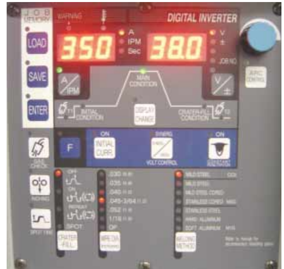
DM350 Key Pad Operation Panel
