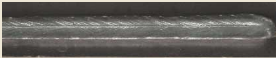
1/8" (3.2 mm) Mild Steel Fillet Weld with .045" (1.2 mm) E70S-3 Mild Steel Wire at 64 in./min.
